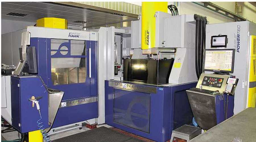
Mould maker Imoplastic in Marinha Grande is taking advantage of an OPS Ingersoll Mold-Centre, consisting of a Gantry Eagle 800 EDM, a Speed Hawk 550 HSC 5-axis machine, as well as an Eagle Powertec generator.
