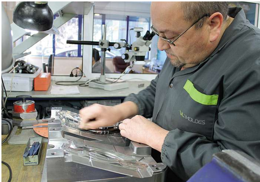
For some moulds, manual polishing is still an important process. However, automated and streamlined processes at Marinha Grande-based VL Moldes has eliminated a lot of manual work.
